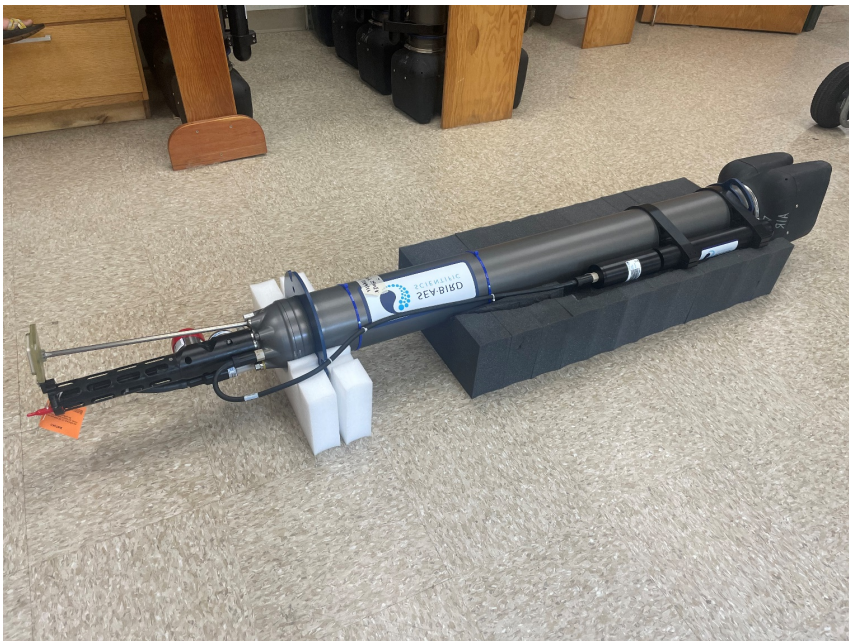
Figure 2: Navis float set on top of foam for sensor cleaning.
