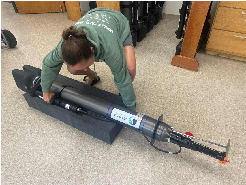
Figure 1: How to properly lift Navis float.
